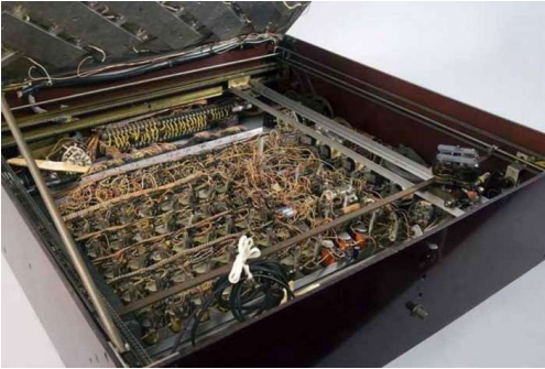
These relay switches underneath the floor of the maze serve as the “brain” for Theseus, the maze-solving mouse.
